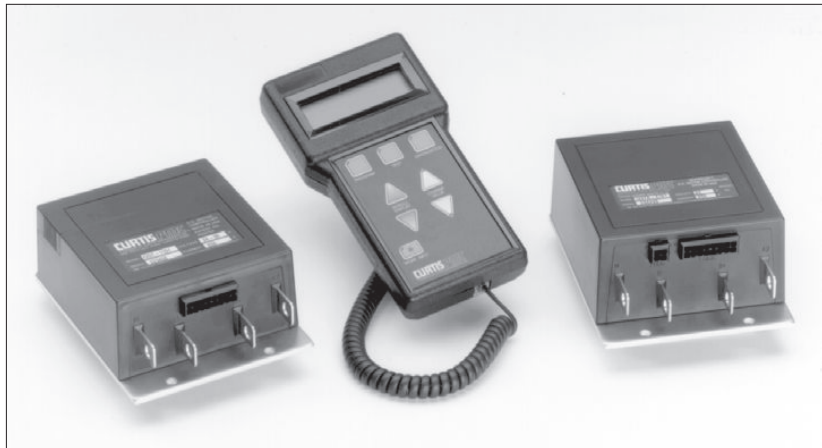
Fig. 1 Curtis PMC 1207 and 1207A electronic motor controllers and handheld programmer.
